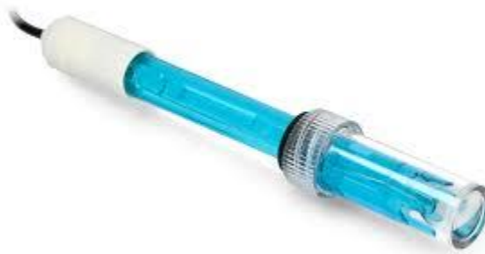
Figure 11 - pH sensor with cap.
